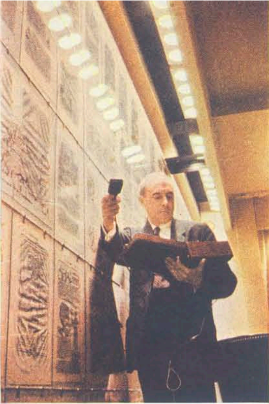
In his New York apartment, Richard Kelly tests the intensity of lamps that "wash" the walls with light.
