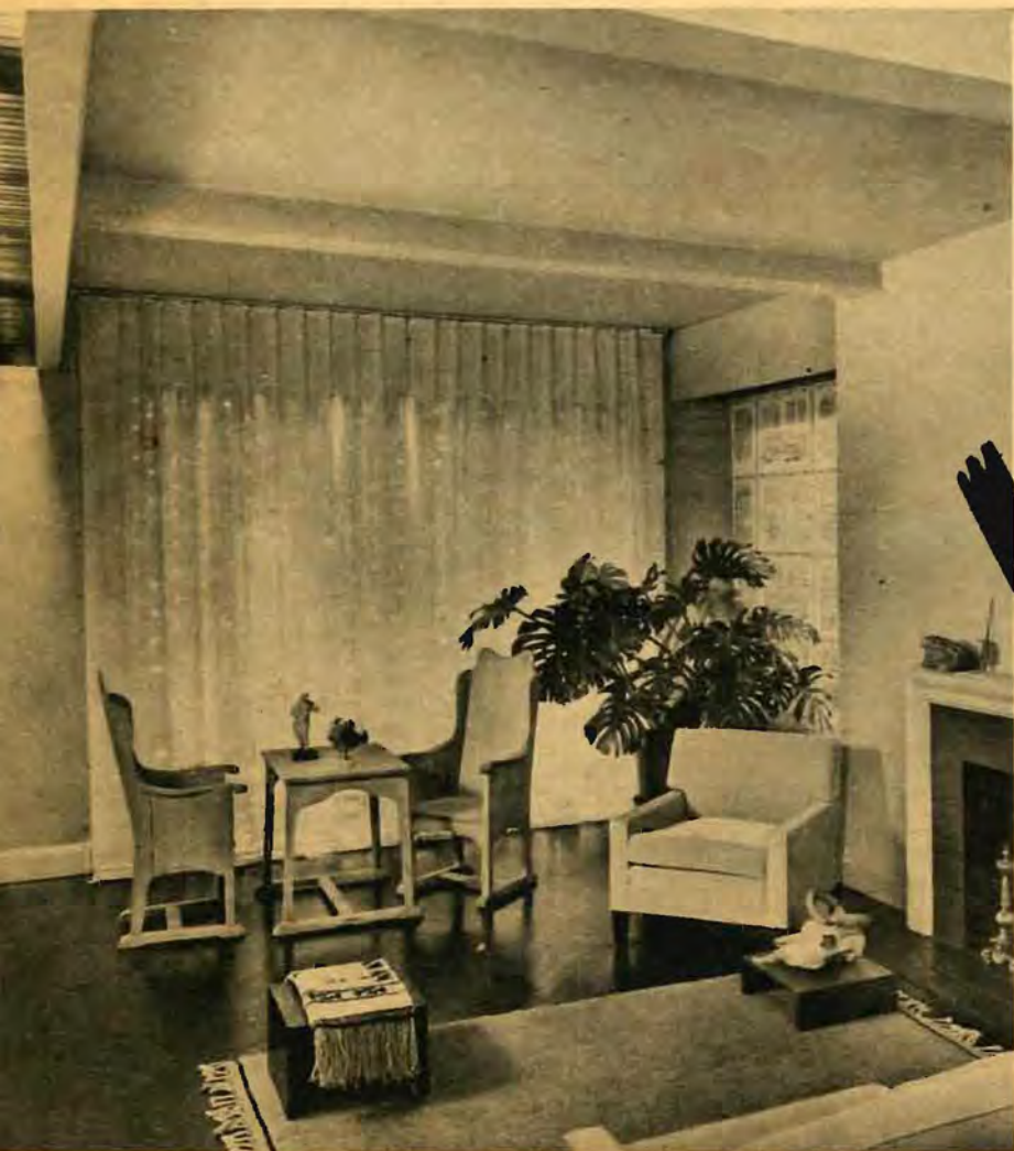
ILLUMINATED DRAPERY throws a radiant net of tiny lights across the living room windows at night. The drapery is a loosely woven material, pierced with minute bulbs that are secured to electrified brass strips on the fabric's reverse side. This experimental, but fire-safe, lighting device may be ordered from Edison Price. Louvered strip, top left, is the shielded underside of a lighting cornice that illuminates a picture wall.
